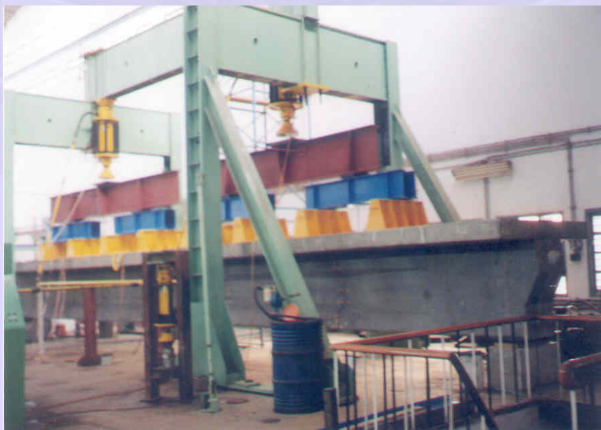
Figure 3-6.6 Set-up for testing a bridge girder
