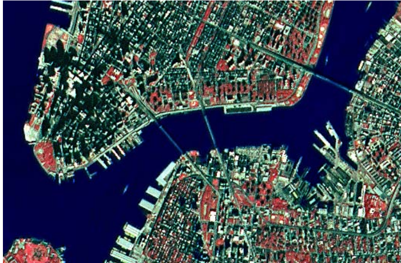
Figure 2e-7: SPOT false-color image of the southern portion of Manhattan Island and part of Long Island, New York. The bridges on the image are (left to right): Brooklyn Bridge, Manhattan Bridge, and the Williamsburg Bridge. (Source: SPOT Image).
